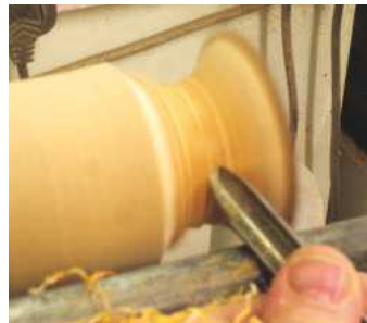
▲ Pic.6 After sanding the inside of the bowl start taking the wood down on the outside to match the shape on the inside, using the bevel rubbing cut applied to the mushroom
